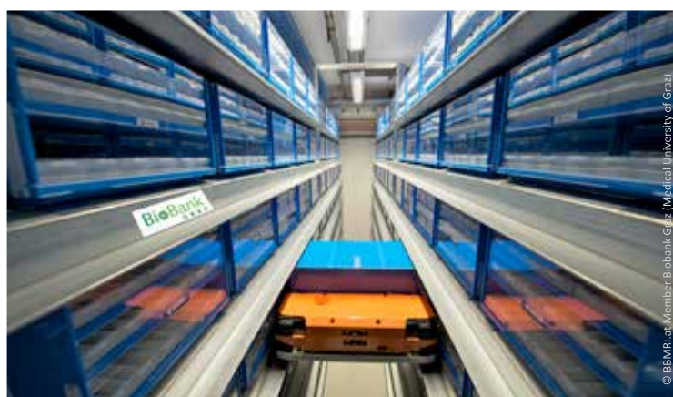
YLOG semi-automated storage system for FFPE samples at Biobank Graz. Biobank Graz currently has 7.5 million samples of which the vast majority is FFPE samples.
