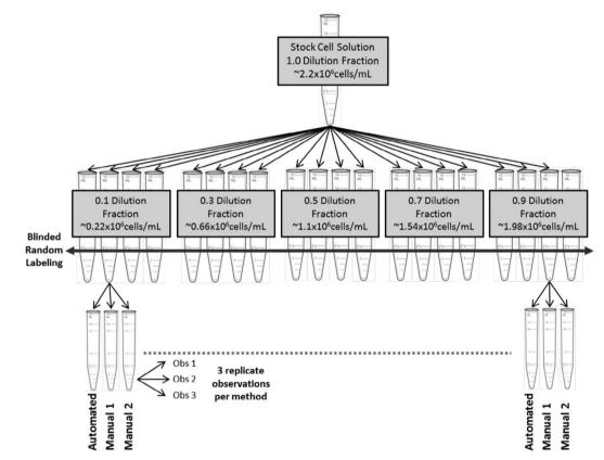
Figure 2. Schematic representation of the cell counting dilution series study experimental design.
